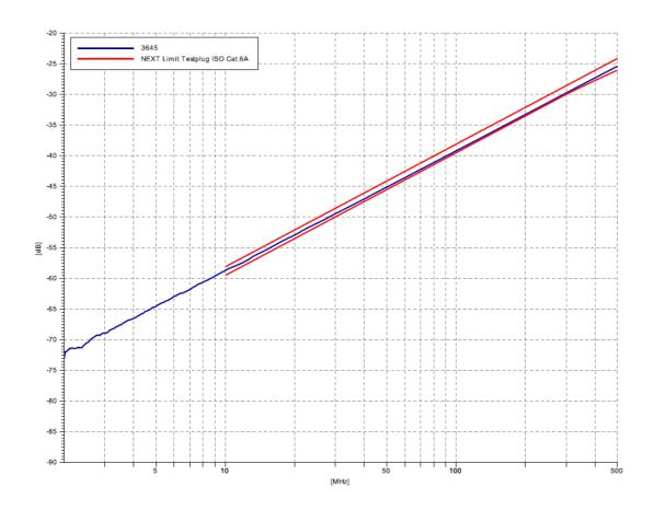
Notice that here the limits of the test are the limits of the Test Free Connectors (TFCs) according to IEC 60512-27-100.
