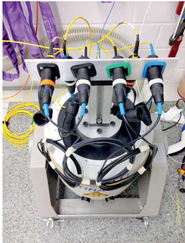
figure 2.b: : Vibration equipment and test cable arrangement
