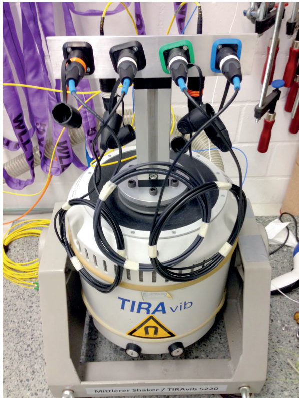
figure 2.a: : Vibration equipment and test cable arrangement
