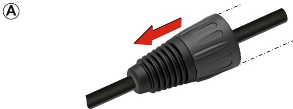
**A** Slide the boot onto the cable.
