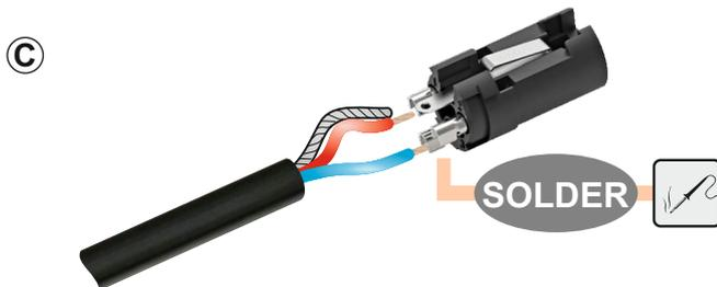
**C** Insert wires into the terminals and solder them.
