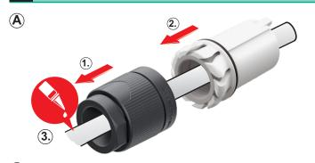
Place the bushing (1) and chuck (2) over the cable.
